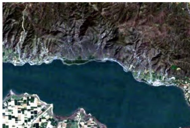
Figure 22. An example of geometric distortion. The procedure of selecting the AOI has initially failed, due to an error of the original image geocoding by several km. Such errors have been corrected, via orthorectification of the original image.
