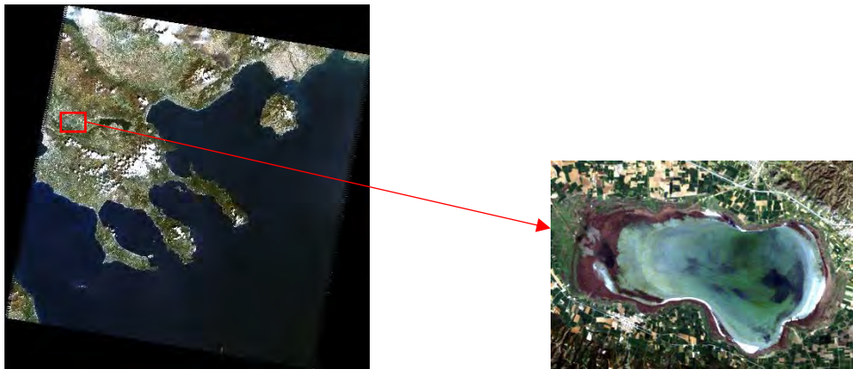
Figure 21. An example of cropping a Landsat TM image (LT51830322008091ESA00) to the AOI. The initial dimension of 7308*6944 pixels was restricted to 403*269 pixels.
