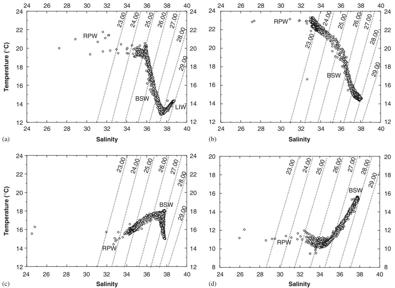
Fig. 3.  $T$ – $S$  diagrams for water mass identification in Strymonikos and Ierissos Gulfs, as measured at CTD stations, during (a) June 1997, (b) September 1997, (c) November 1997 and (d) February 1998. Dashed lines indicate  $\sigma_t$  lines.
