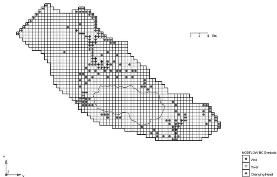
Fig. 8 Finite difference grid and boundary conditions of the study area
