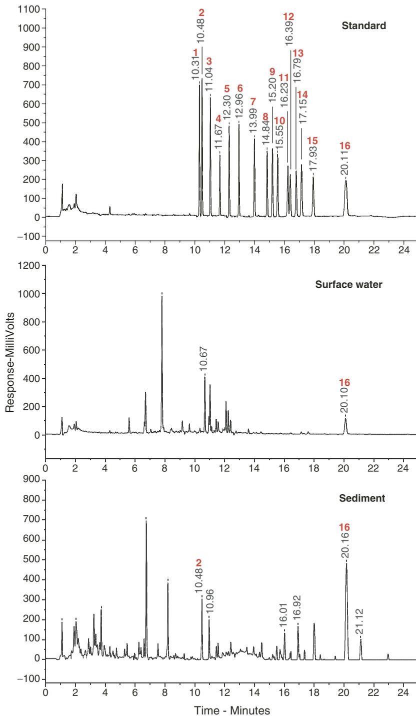
Figure 2. GC chromatograms of pesticides detected by ECD. (Top) GC-ECD chromatogram of a standard solution of 16 pesticides, as listed in table 1, dissolved in hexane at a concentration of 50  $\mu\text{g/L}$ . (Bottom) GC-ECD chromatograms of surface-water extract (middle) and a sediment-sample extract.
