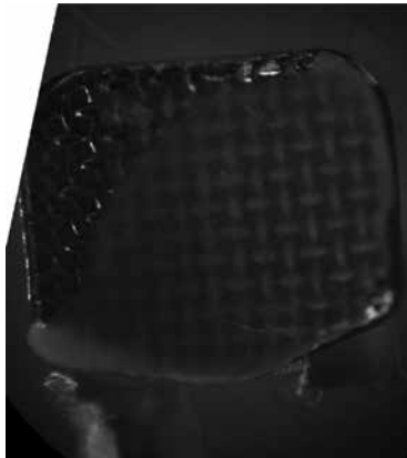
Fig. 2. Bracket base ARI score = 1, seen at 20× magnification
